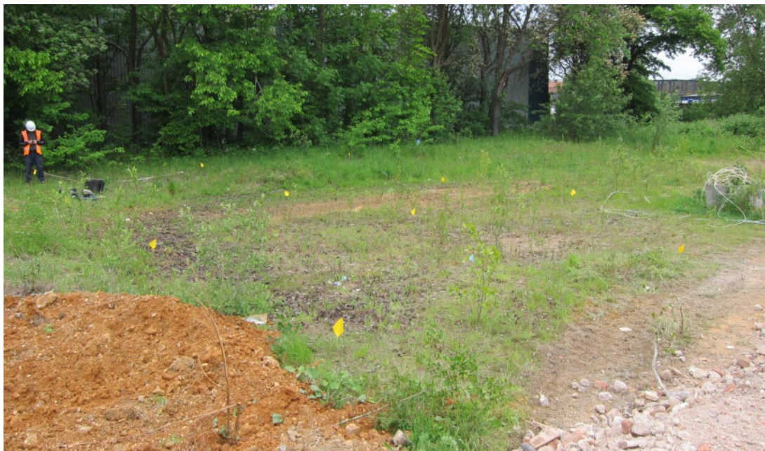
Photograph 13-2: Laying out of SVS grid across the remediation area
