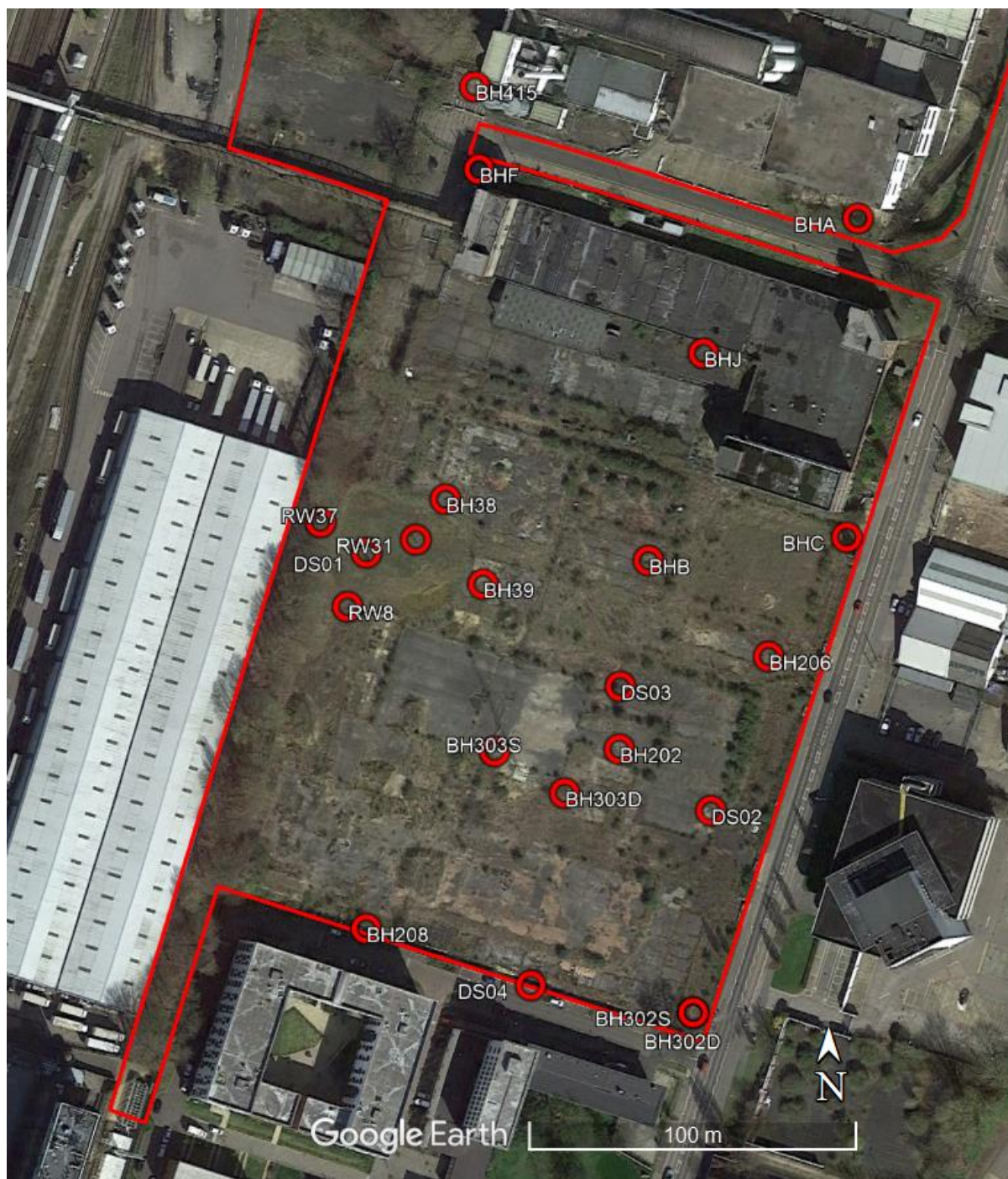
Figure 6-1: Groundwater wells monitored during September 2017
