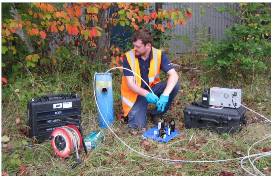
Photograph 6-3: Groundwater sampling using low-flow bladder pump
