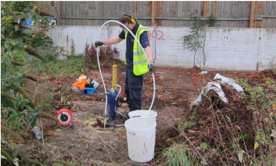
Photograph 6-2: Groundwater well purging through use of HDPE tubing and Power-pack
