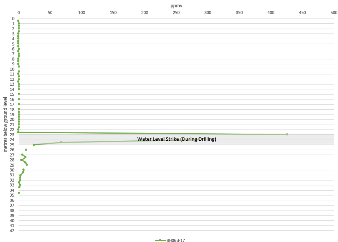
Figure 7-7: PID profile associated with BH06d-17 (0.5 m to 40 m bgl)
