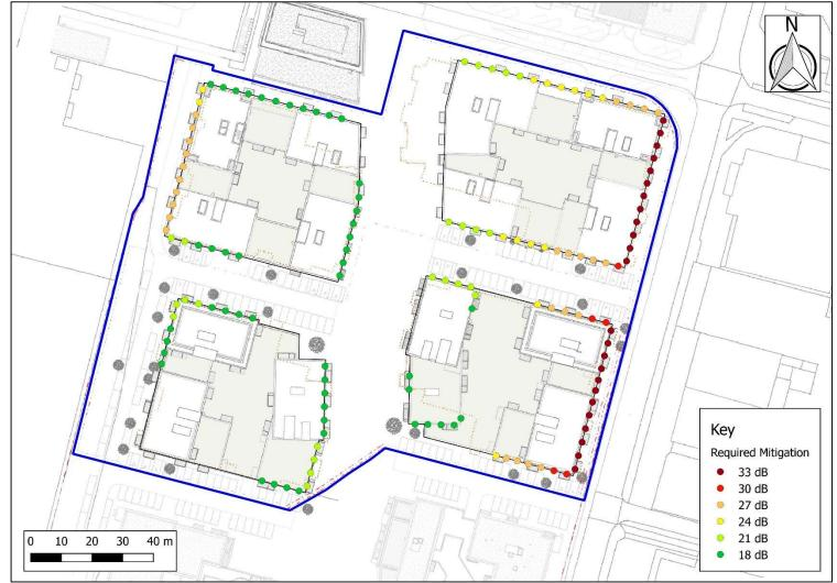
Appendix 10.6: Calculated Façade Reduction Requirements (R<sub>w</sub> + C<sub>tr</sub>), First Floor
