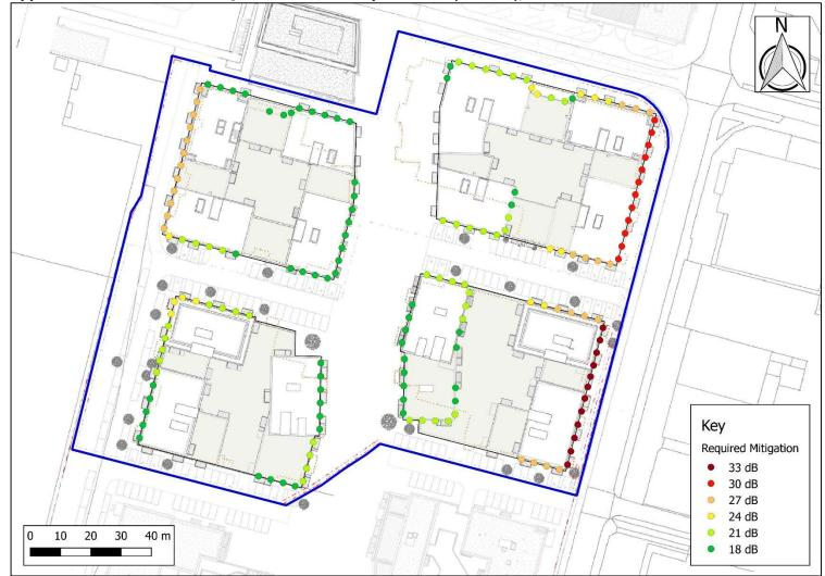
Appendix 10.10: Calculated Façade Reduction Requirements (R<sub>w</sub> + C<sub>tr</sub>), Fifth Floor
