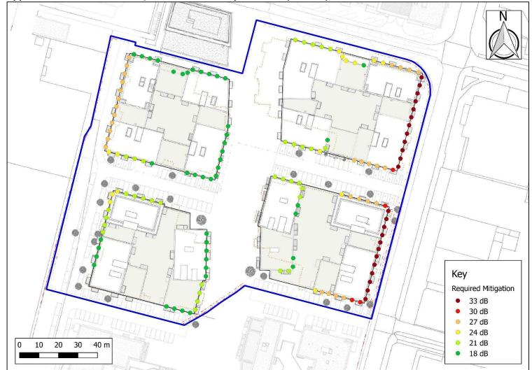
Appendix 10.8: Calculated Façade Reduction Requirements (R<sub>w</sub> + C<sub>tr</sub>), Third Floor
