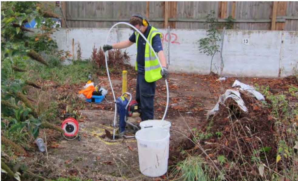
Photograph 6-1: Groundwater well purging through use of HDPE tubing and Power-pack
