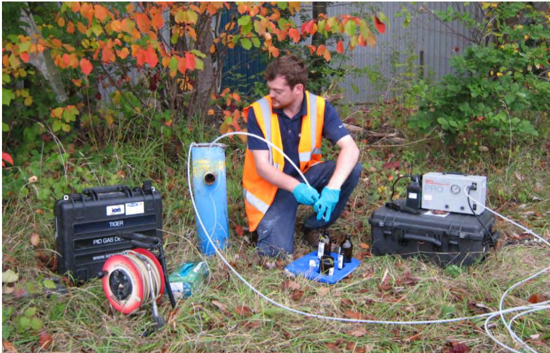
Photograph 6-2: Groundwater sampling using low-flow bladder pump
