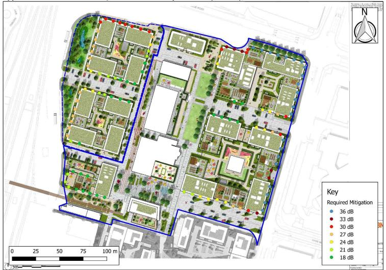
Appendix 10.11: Calculated Façade Reduction Requirements (R<sub>w</sub> + C<sub>tr</sub>), Second Floor
