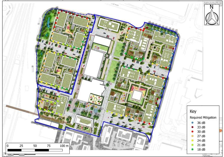
Appendix 10.13: Calculated Façade Reduction Requirements (R<sub>w</sub> + C<sub>tr</sub>), Fourth Floor
