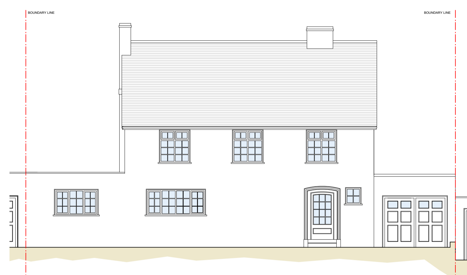
EXISTING FRONT ELEVATION 1:100 SCALE
