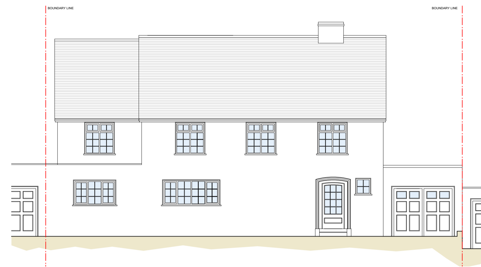
PROPOSED FRONT ELEVATION - 1:100 SCALE
