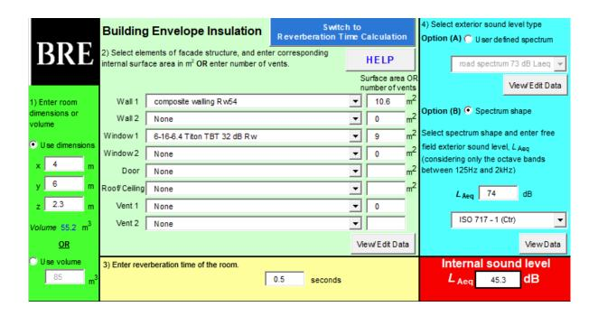
This shows that with a Triton TBT window with double glazing configuration of 6mm glass/16mm cavity/ 6.4mm acoustic laminated glass (laboratory tests data sheet at rear of this report)<sup>4</sup> with a laboratory measured sound insulation performance of 32 (-1:-3)  $R_w(C;C_{tr})$  dB the expected internal sound level with a 74 dB  $L_{amax,regular}$  event outside will be 45 dB inside and thus equal the required criteria.
