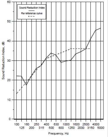
Rating according to BS EN ISO 717-1:1997 Rw(C;Ctr)= 32 (-1;-3) dB \* shows measurement corrected for background # shows limit of measurement due to background + shows frequency beyond standard and not UKAS accredited
