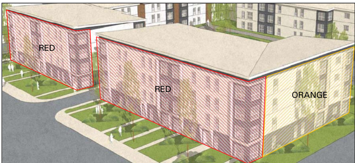
Figure 2 – Front Aspect with Coloured Zones for Sound Insulation
