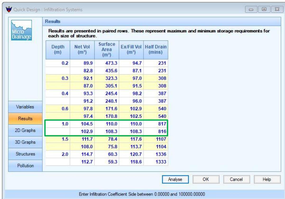
**Figure 4.4 – Catchment A-Half Drain Time Calculation Results**
