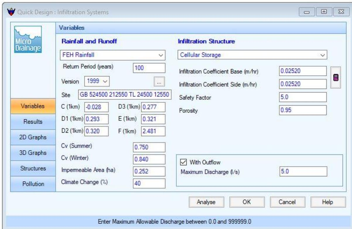
Figure 4.16 – Catchment B-Half Drain Time Calculation with 5 l/s Discharge Variables
