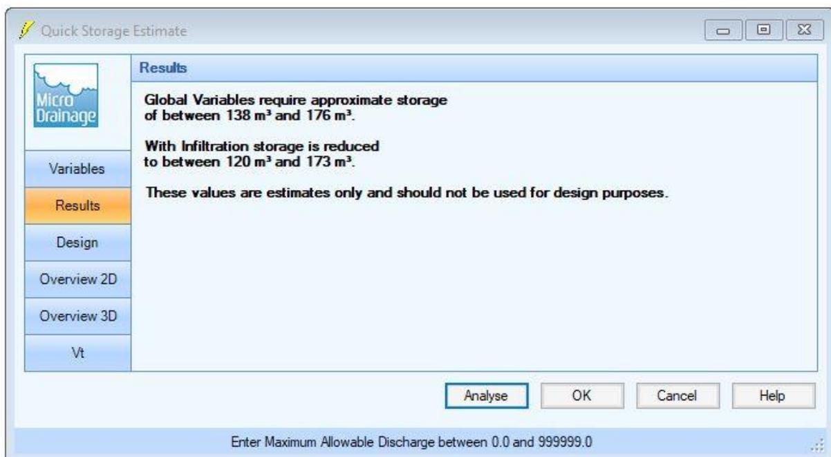
Figure 4.15 – Catchment B-Quick Storage Estimate with 5 l/s Discharge Results
