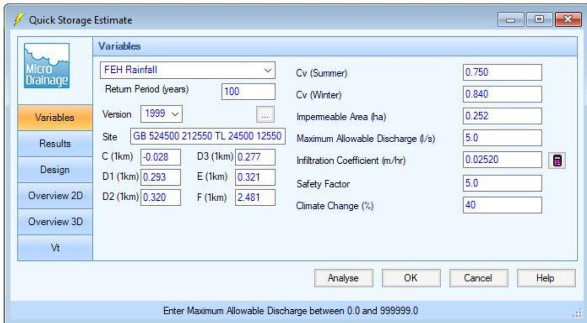
Figure 4.14 – Catchment B-Quick Storage Estimate with 5 l/s Discharge Variables
