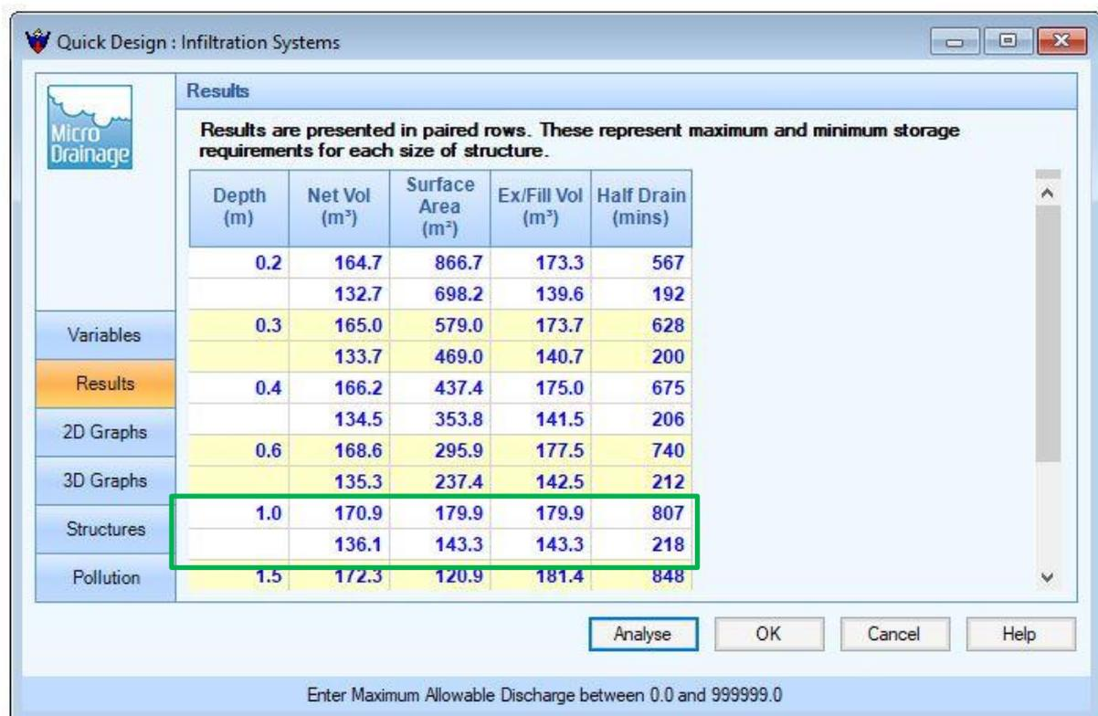
Figure 4.17 – Catchment B-Half Drain Time Calculation with 5 l/s Discharge Results
