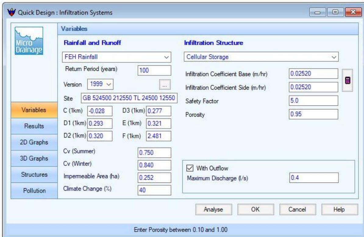
Figure 4.12 – Catchment B-Half Drain Time Calculation with Greenfield Rate Discharge Variables
