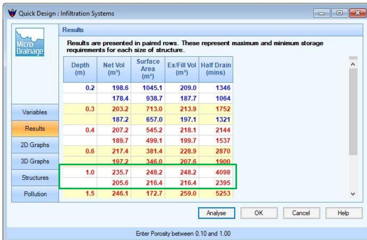
Figure 4.13 – Catchment B-Half Drain Time Calculation with Greenfield Rate Discharge Results
