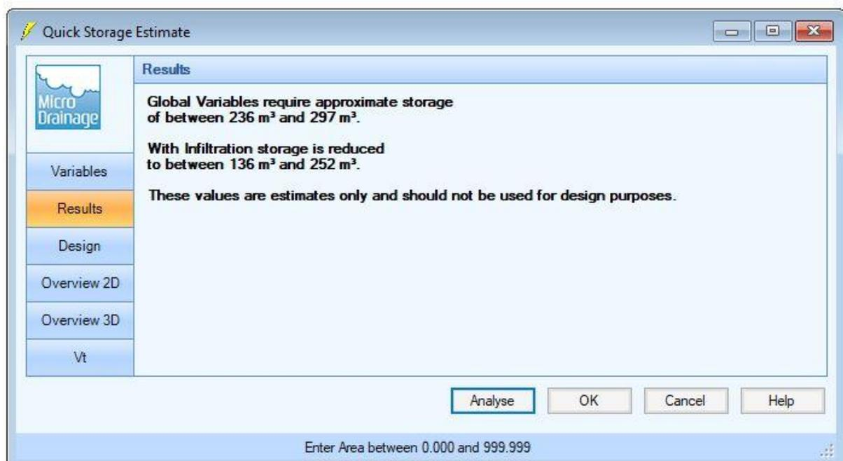
Figure 4.11 – Catchment B-Quick Storage Estimate with Greenfield Rate Discharge Results
