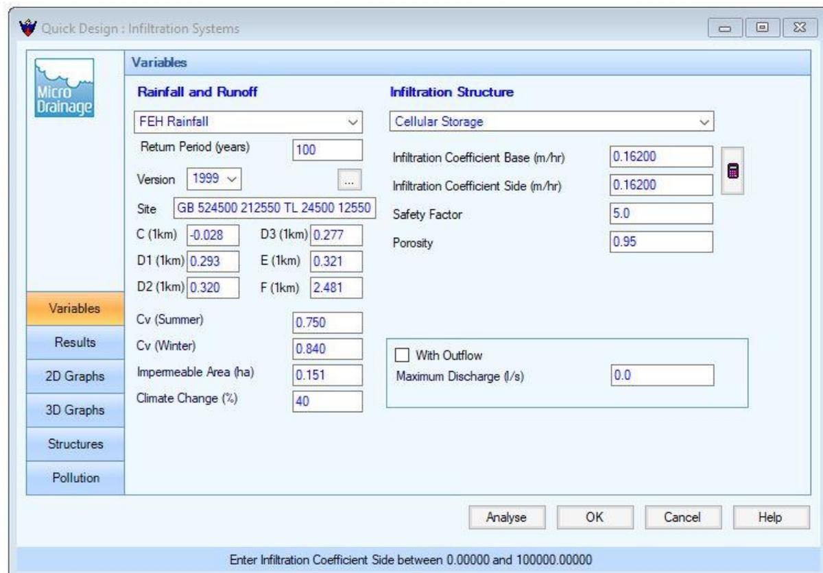
**Figure 4.3 – Catchment A-Half Drain Time Calculation Variables**
