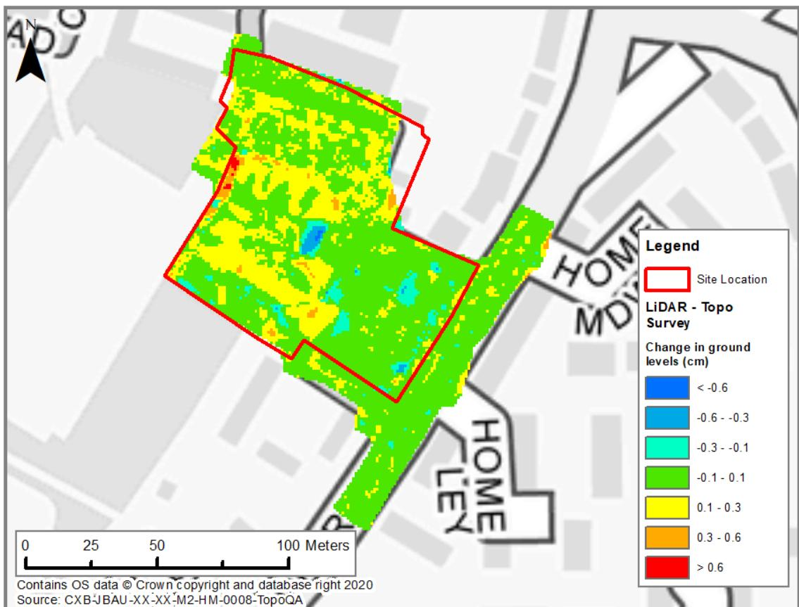
**Figure C-1: Topographic survey vs LiDAR**
