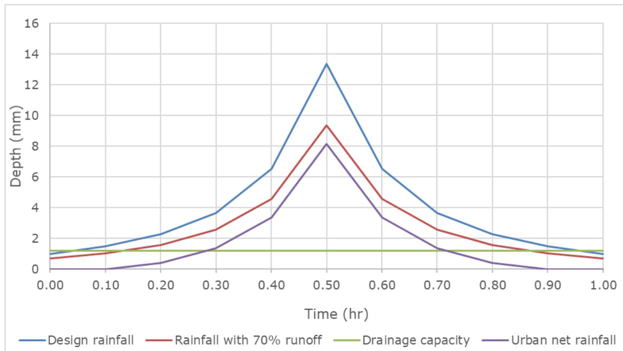
Figure 3-2: Graph illustrating the stages in hyetograph calculations, demonstrated using the 100-year, 1-hour storm.
