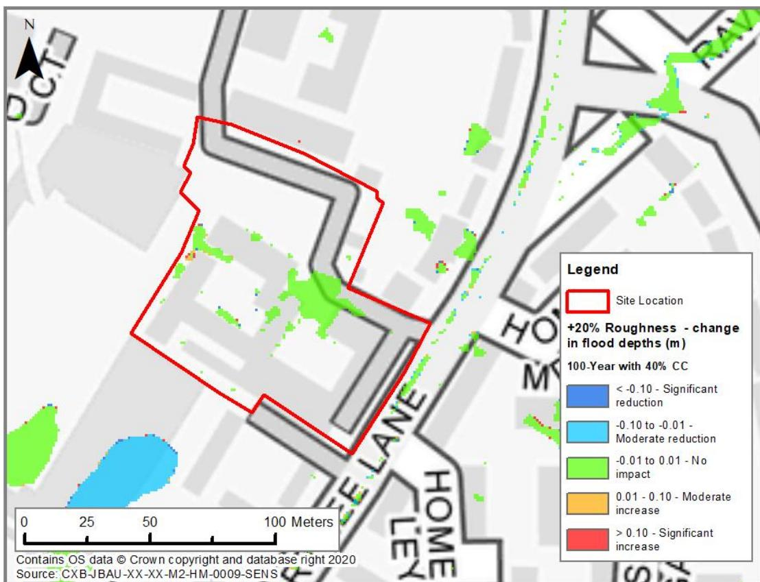
**Figure E-2: Sensitivity to an increase in roughness**
