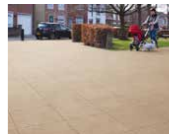
Area: Private amenity Type: Concrete Flags Size: 400x400mm Colour: Natural
