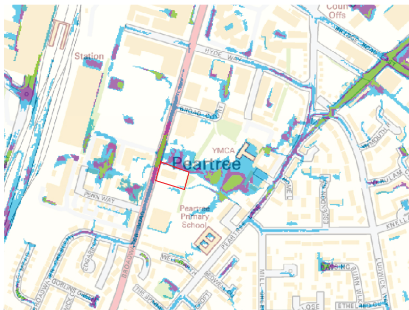
Figure 2: Risk of surface water flooding to the site as taken from the 2016 SFRA [9] . The blue shaded areas are denoted as areas with between a 1 in 100 and 1 in 1000 yr risk of SW flooding in any one year - the equivalent of EA Flood Zone 2. The purple shaded denote areas with risk between 1 in 30 and 1 in 100 yr (EA Flood zone 3).
