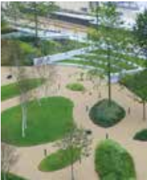
Area: Podium gardens Type: Addastone resin bonded gravel Size: 6mm aggregate size Colour: Buff
