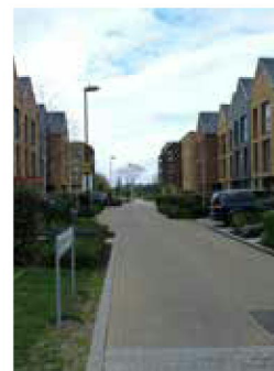
Shared surface treatment
