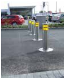
Area: Hyde Way Type: Rising bollard
