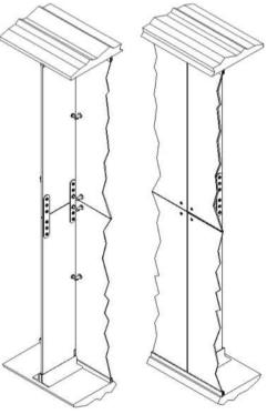
Typical detail of a planar glazing system, with structural fins in glass. Final details to specialists detail design.
