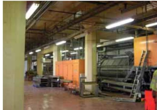
4 The internal structure is designed to support the weight of the original equipment. All the columns and foundations were also designed to provide for future addition of two storeys above the roof.
