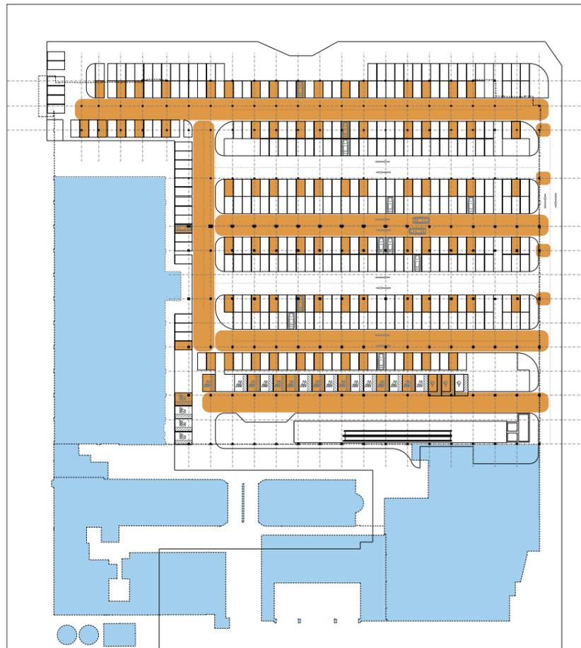
Basement plan showing the parking layout superimposed on the existing column grid
