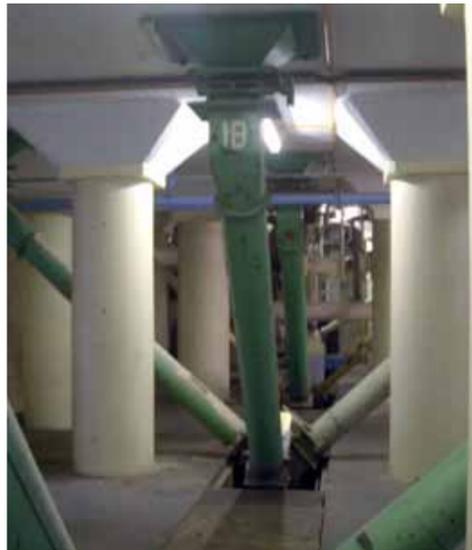
3 Silos discharge the grain into an underground conveyor-belt system
