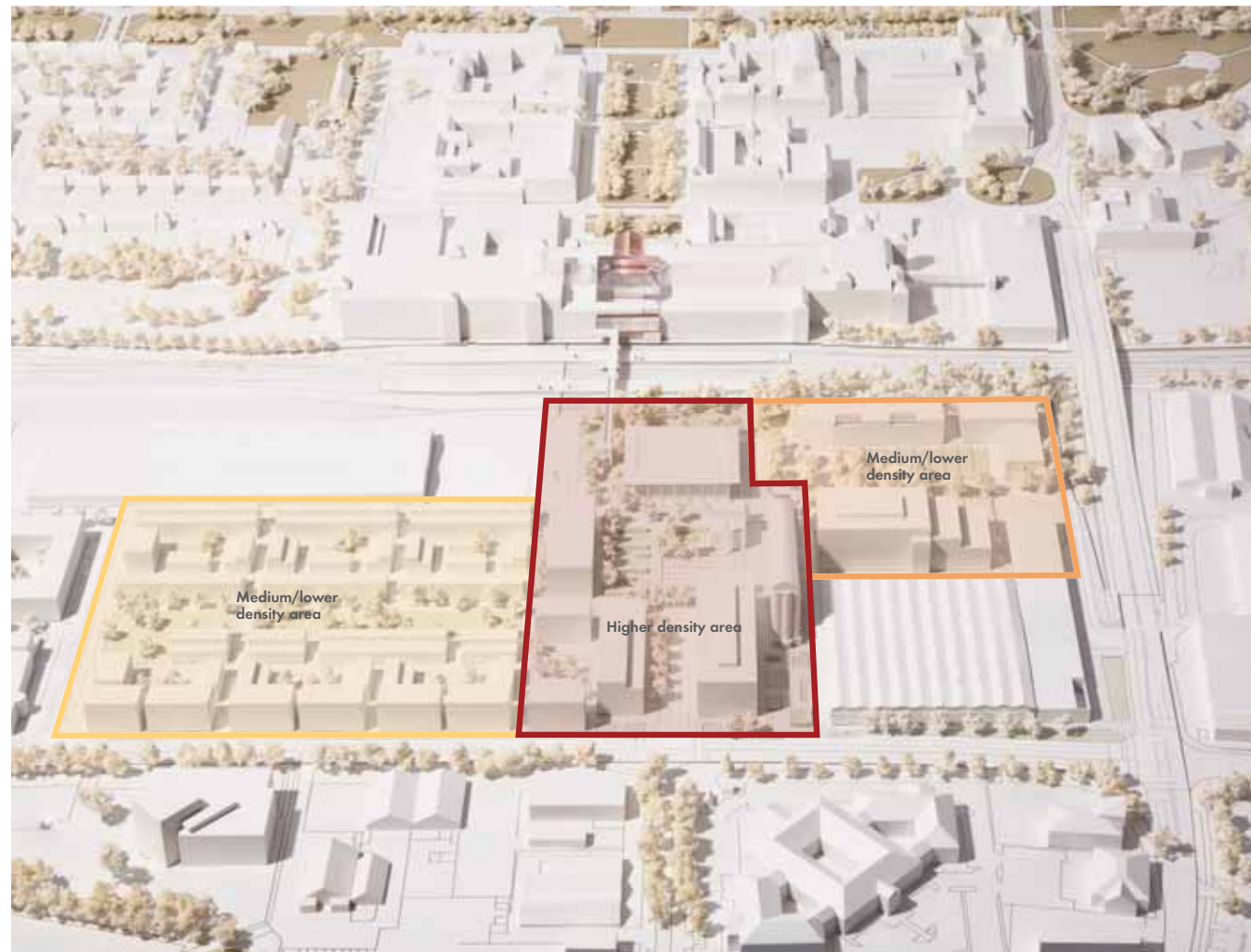
Photograph of sketch model illustrating 3 density and character zones across the site
