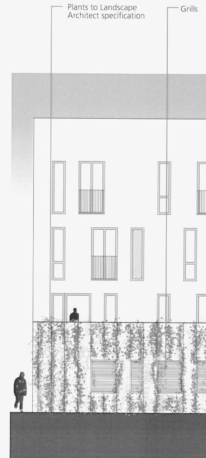
Elevation showing ventilation for parking structure
