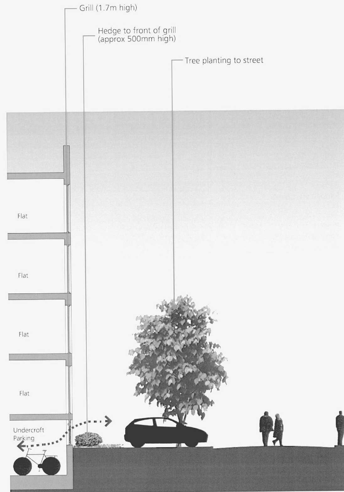
Section showing ventilation for parking structure
