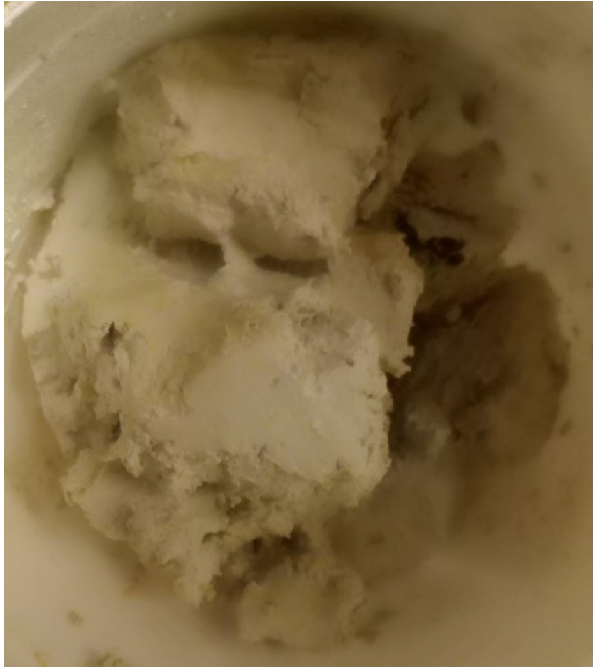
SPT sample from BH02 at 18.0mbgl.
