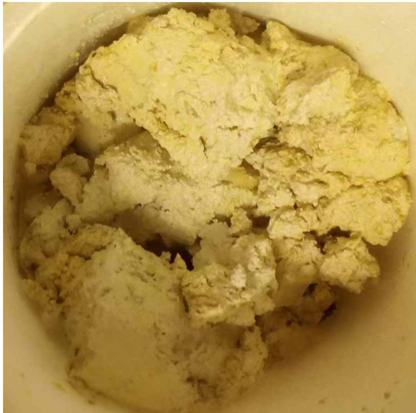
SPT sample from BH03 at 14.0mbgl.
