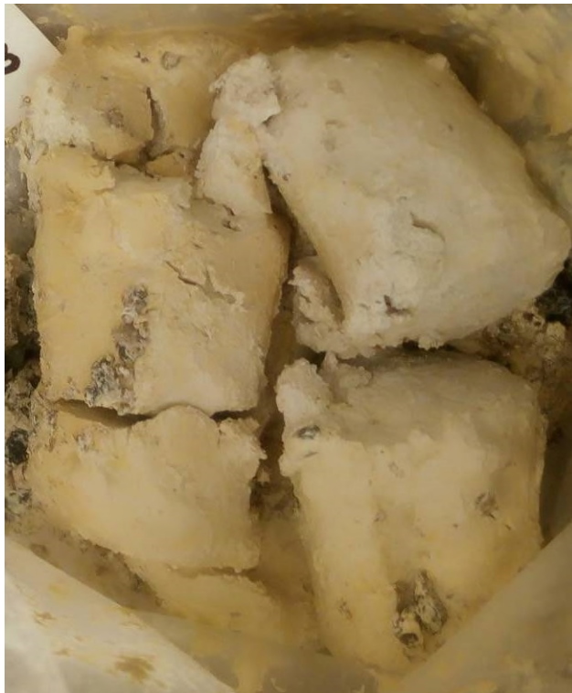
SPT sample from BH03 at 20.0mbgl.
