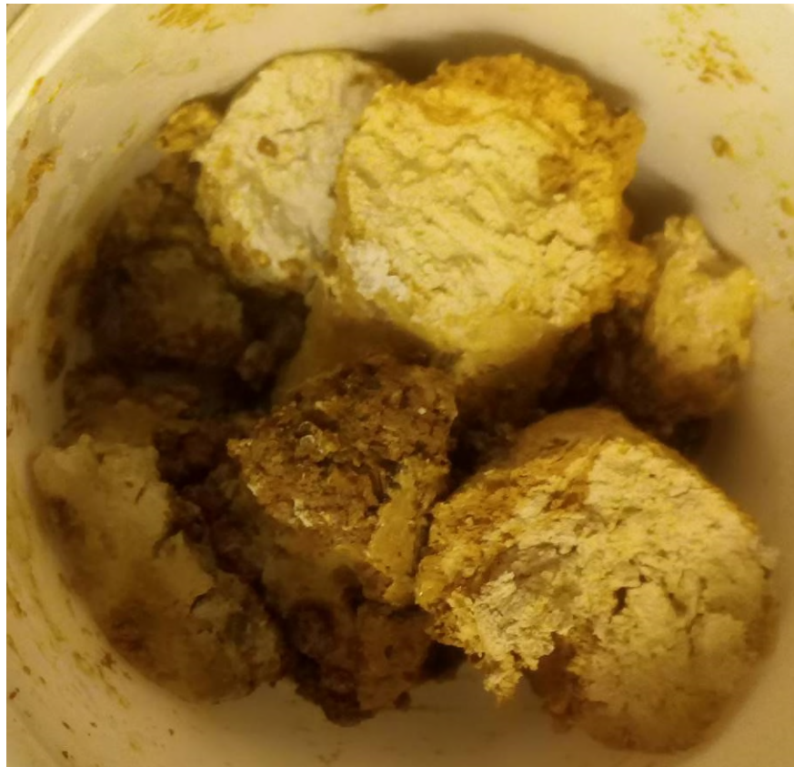
SPT sample from BH03 at 12.0mbgl.
