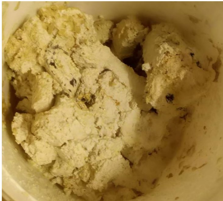
SPT sample from BH02 at 15.0mbgl.
