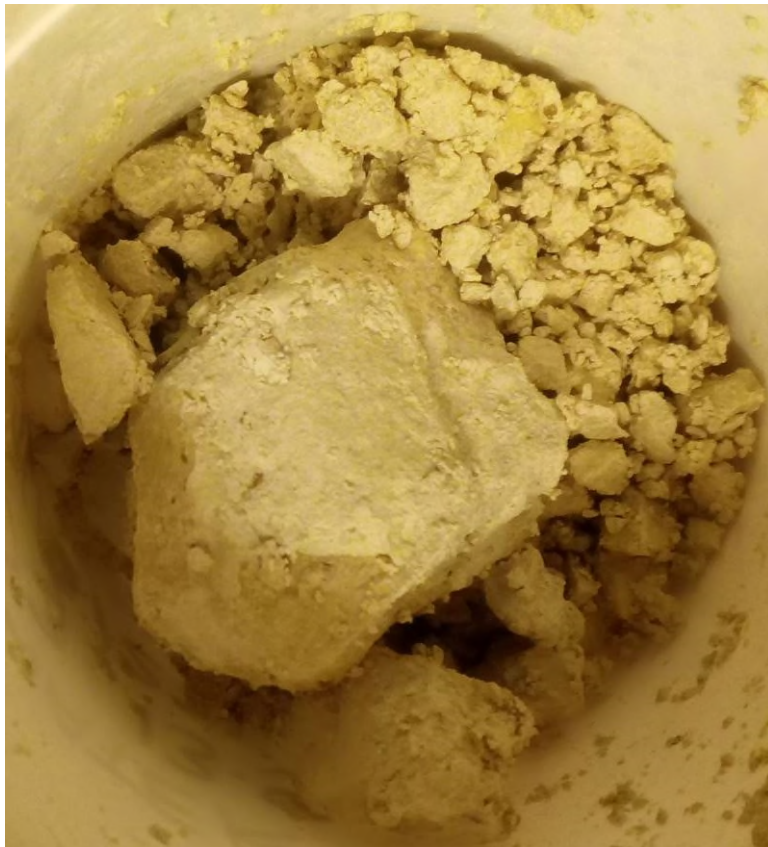
Trimming from UT100 shoe conducted in BH03 at 13.0mbgl.
