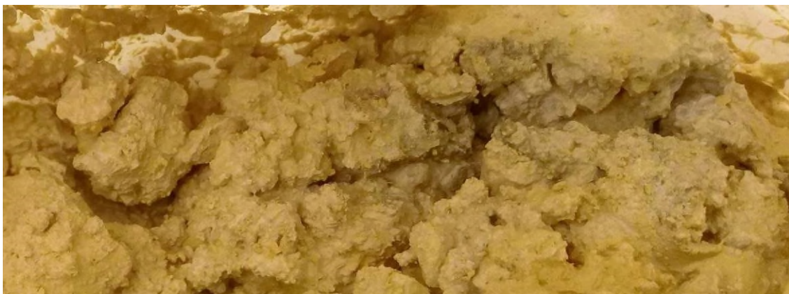
Failed UT100 sample from 19.0-19.2mbgl.
