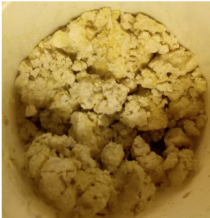
Trimming from UT100 shoe conducted in BH03 at 15.0mbgl.
