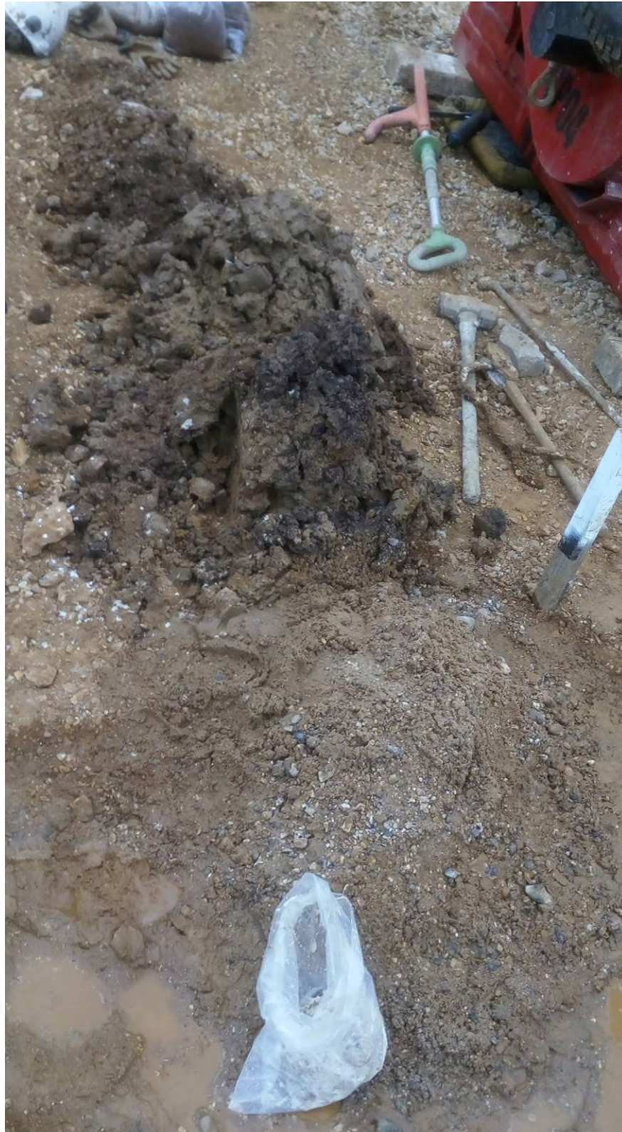
Materials retrieved from the cable percussive borehole at DPSH39 0.0-14.0mbgl.
