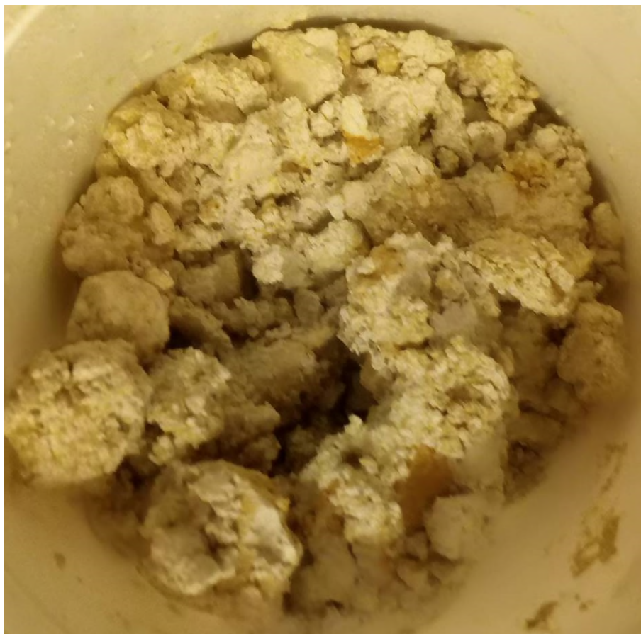
Trimming from the UT100 shoe conducted in BH02 at 14.0mbgl.
