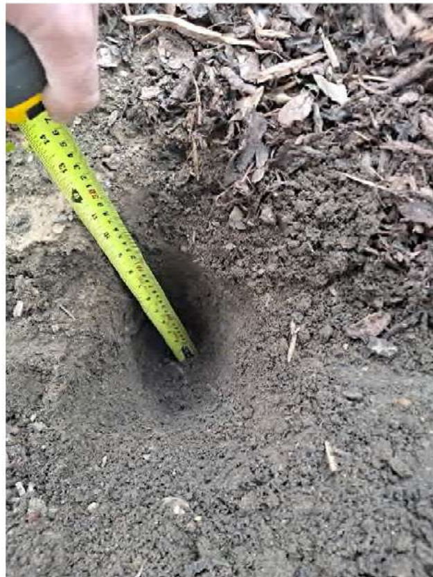
Plate 2. Location 2 (see plan in Appendix A); 300mm of certified clean topsoil
