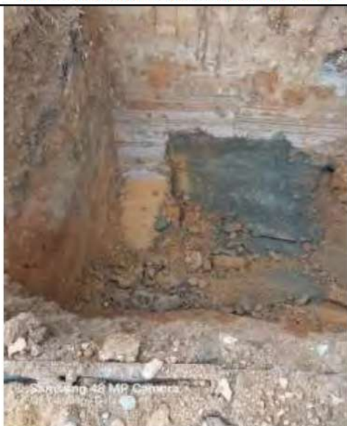
Plate 3. Tainted/stained deep soils east 2.6m
