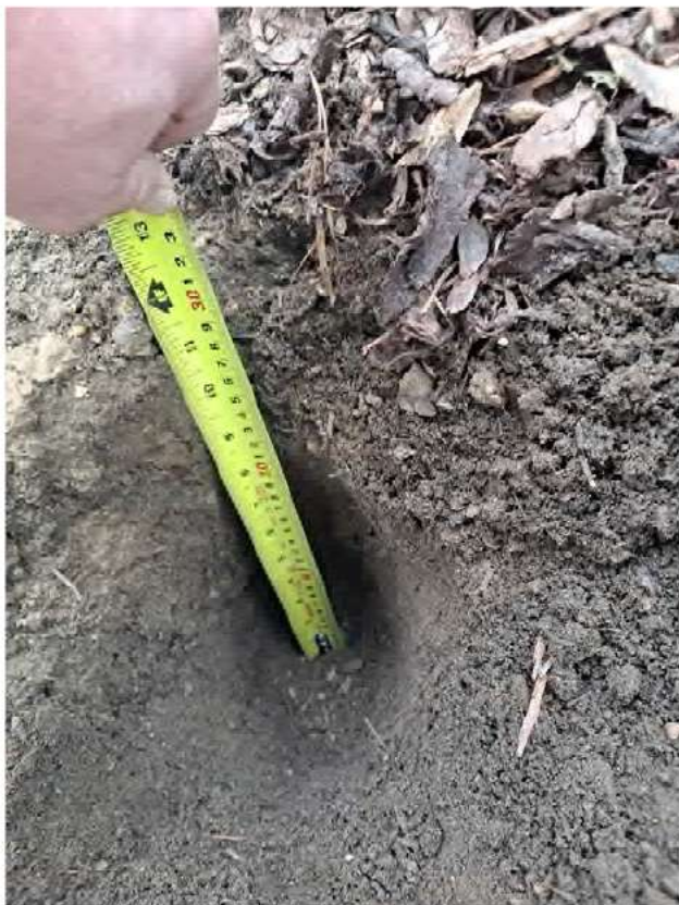
Plate 1. Location 1 (see plan in Appendix A); 300mm of certified clean topsoil
