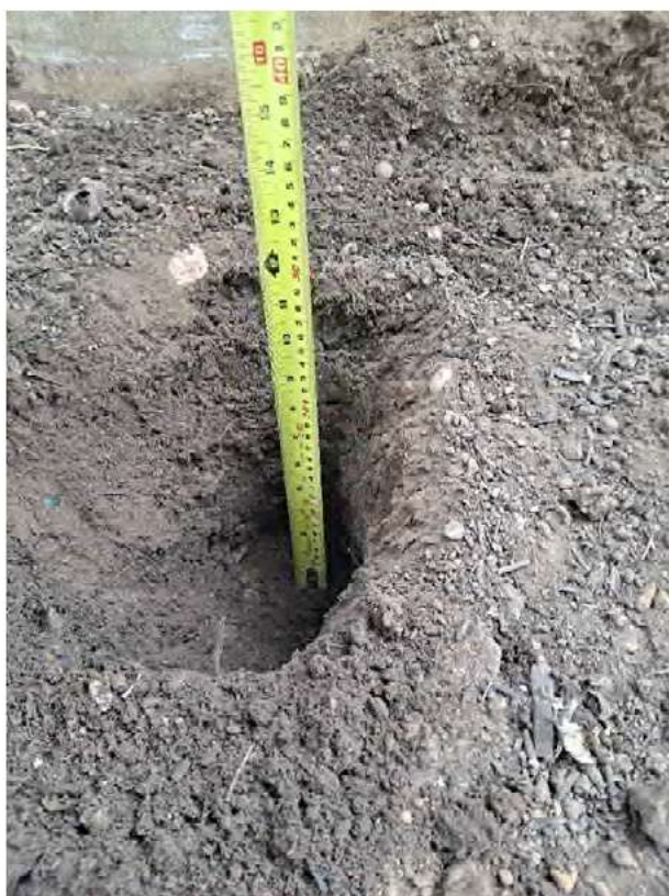
Plate 3. Location 3 (see plan in Appendix A); 300mm of certified clean topsoil
