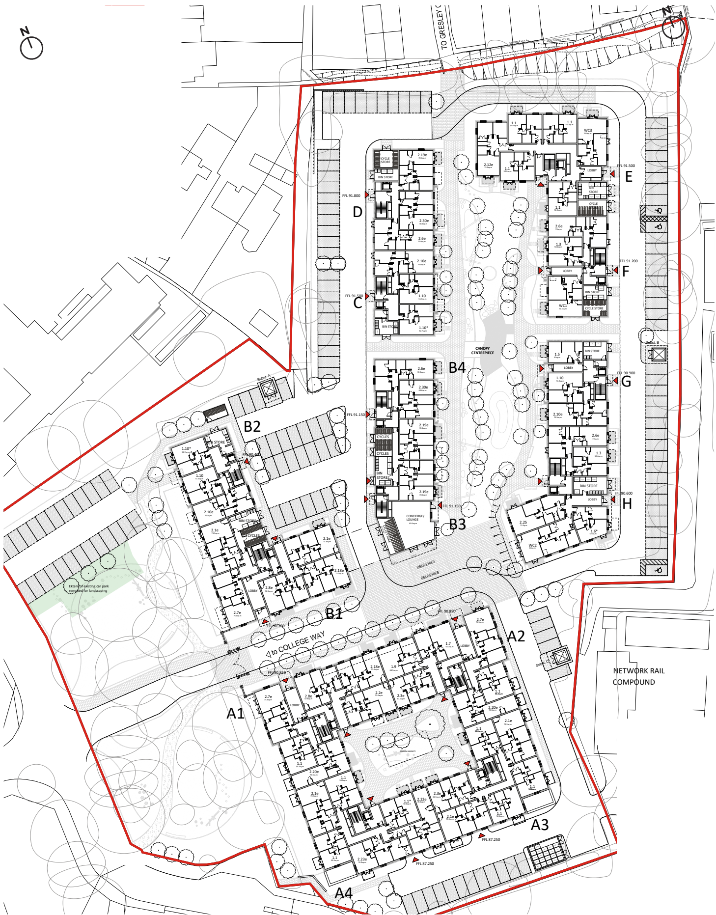
FIG 35 - PROPOSED GROUND FLOOR SITE LAYOUT
