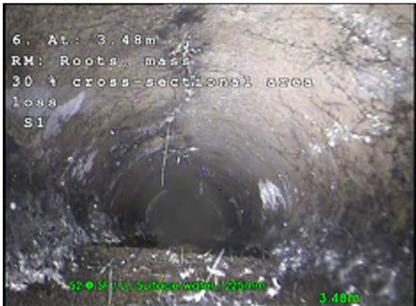
Photo: 37_37_297_A.jpg, 00:00:34 3.48m, Roots, mass 30 % cross-sectional area loss S1
