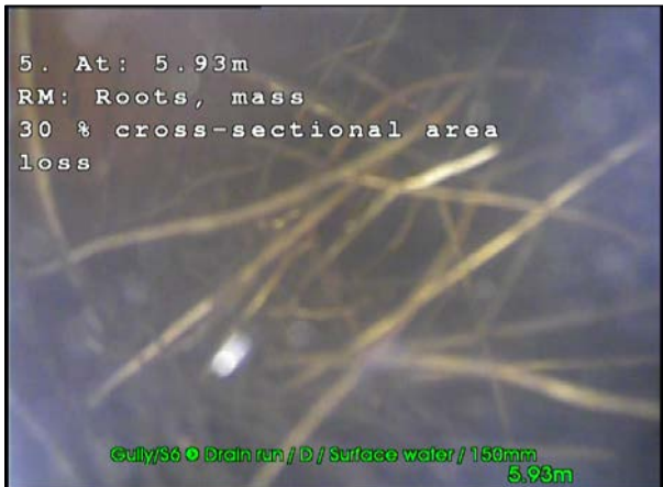
Photo: 17_17_113_A.jpg, 00:01:19 5.93m, Roots, mass 30 % cross-sectional area loss
