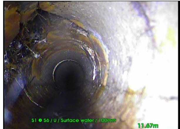
Photo: 22_22_489_A.jpg, 00:01:13 11.67m, Hole in drain/sewer, from 9 to 12 o'clock
