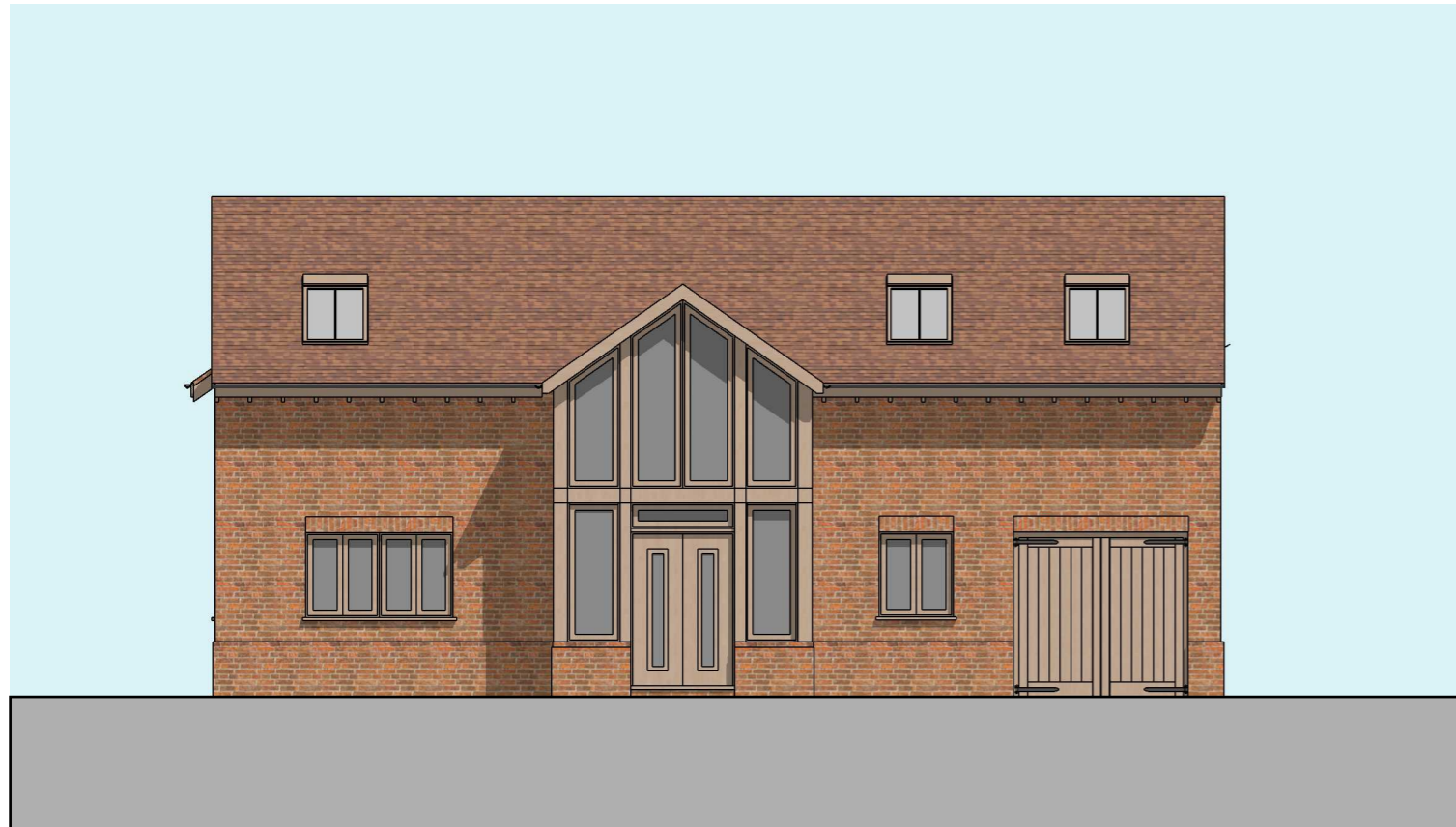
PROPOSED FRONT ELEVATION, SETTLEMENT UNIT 1
