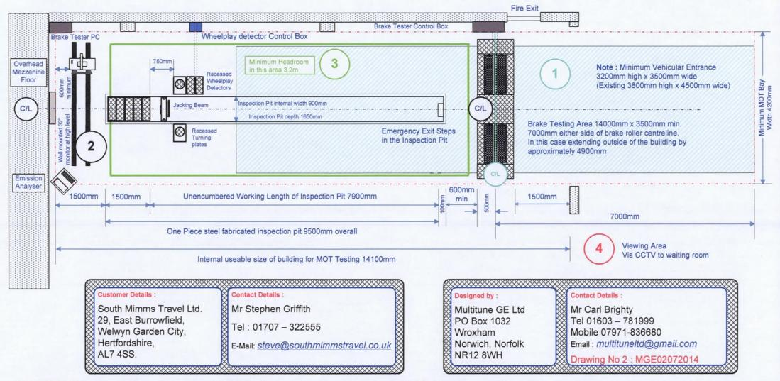
ATL MOT Testing Bay-Class 4, 5L & 7. (Drive in - reverse out) Utilising Inspection Pit.
