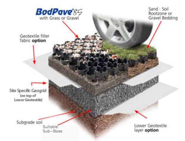
TYPICAL BOD-PAVE CONSTRUCTION SCHEMATIC.
