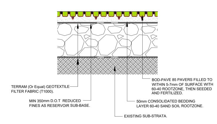
TYP PERMEABLE CONSTRUCTION DETAIL (AT OVERFLOW PARKING AREA).
