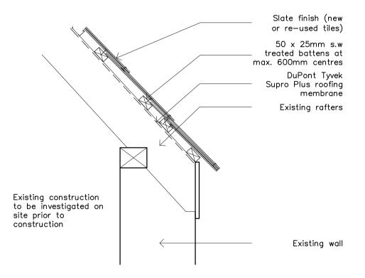
DETAIL 01 - TYPICAL EAVES DETAIL Detail to be amended to suit roof pitches 1:10
