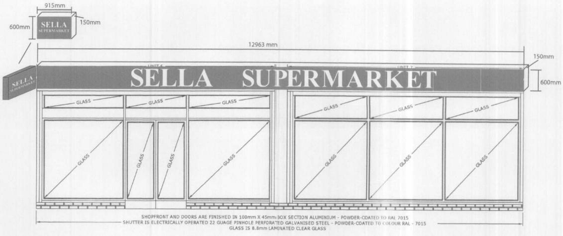
Fascia structure is an Adonised Aluminium box, dimensions 12963mm x 600mm x 150mm
