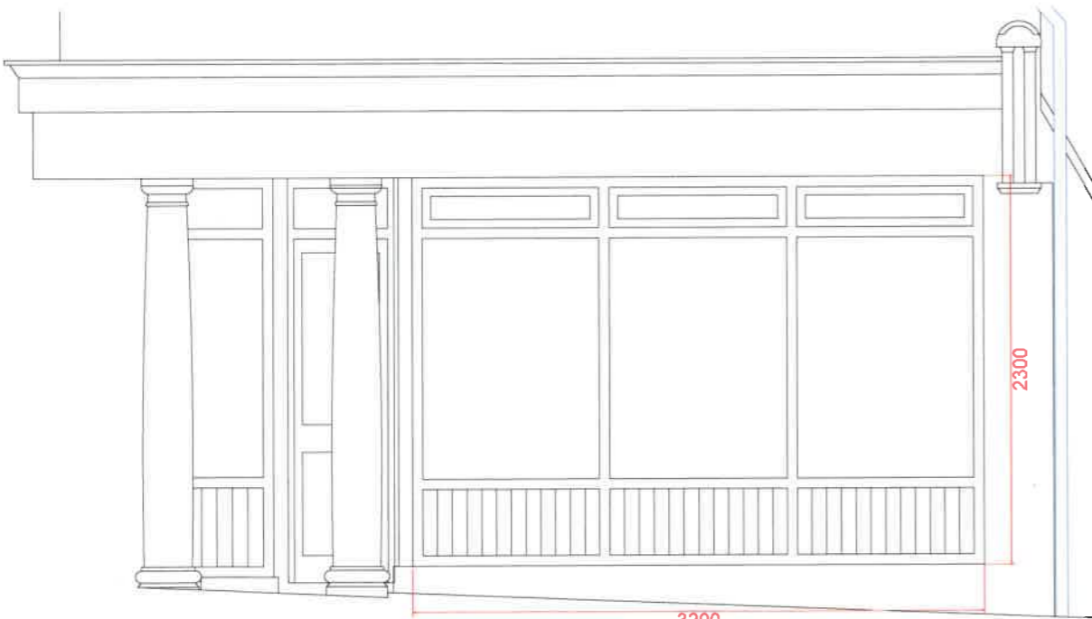
ELEVATION A - SCALE 1:20 MATERIAL : PAINTED SOFTWOOD
