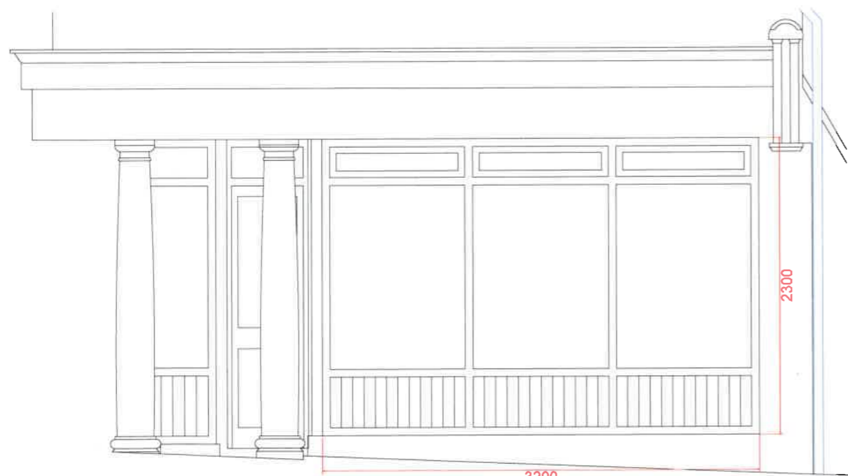
ELEVATION A - SCALE 1:20 MATERIAL : PAINTED SOFTWOOD
