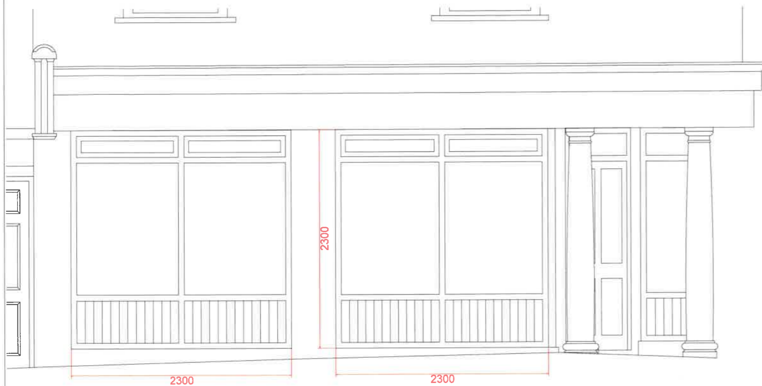
ELEVATION D - SCALE 1:20 MATERIAL : PAINTED SOFTWOOD
