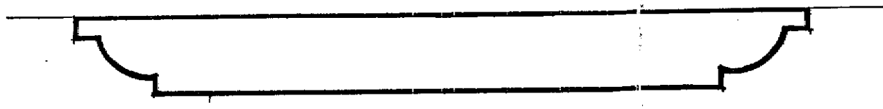
20 MOULDING TO WALL PANELS
