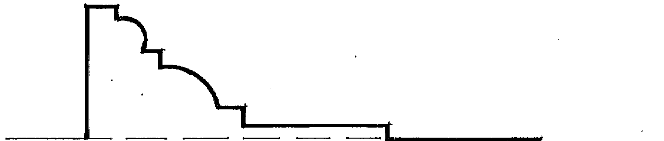
36 ARCHITRAVE TO LARGE ARCH.
