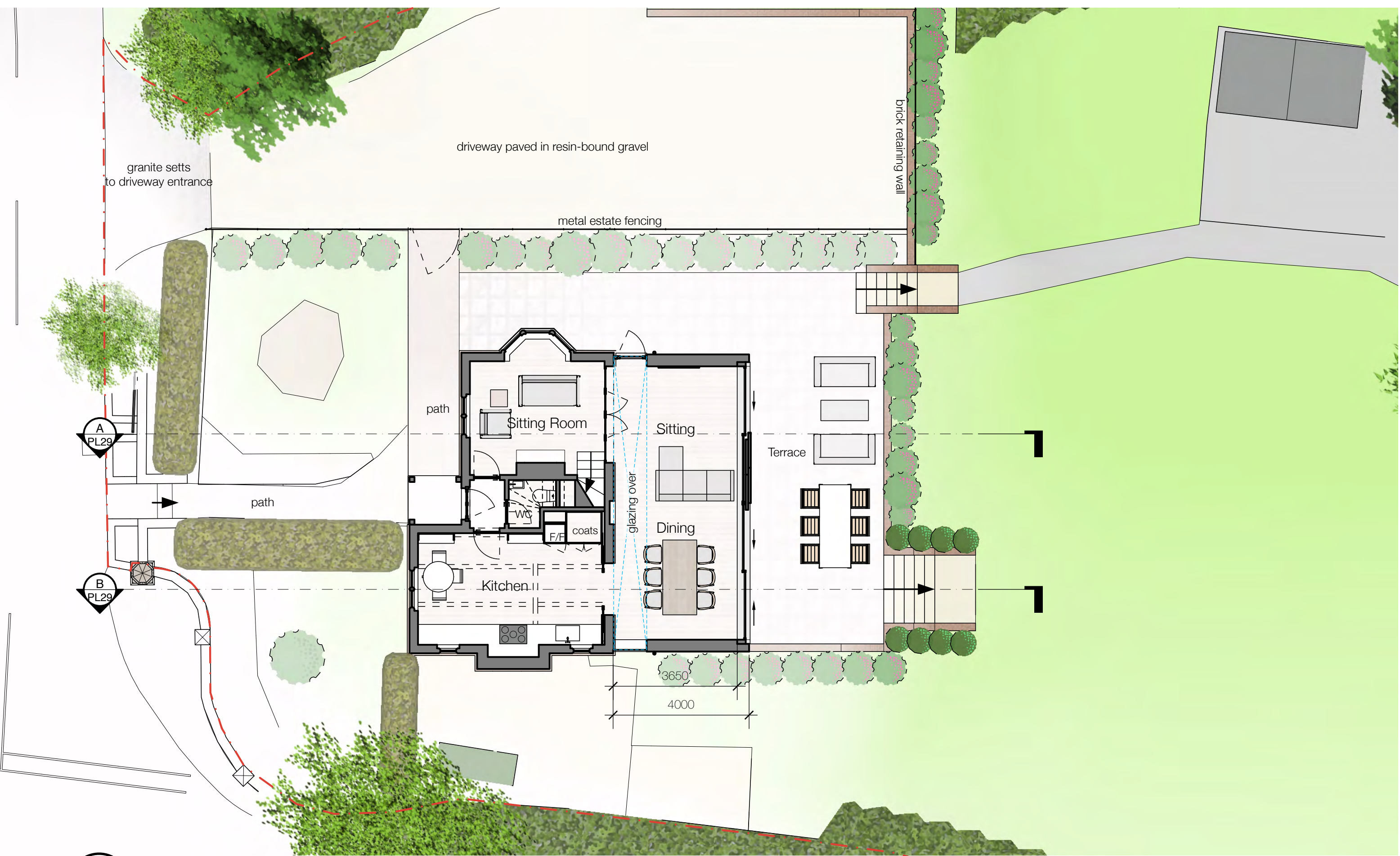
A Proposed Ground Floor Plan PL11 1:100
