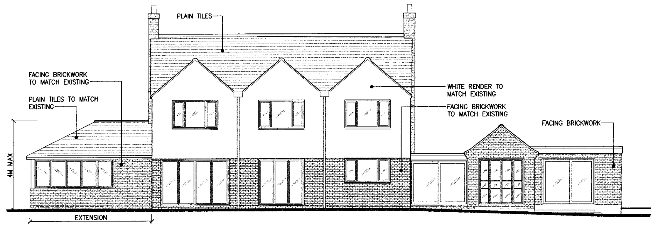
NORTH ELEVATION C SCALE 1:100
