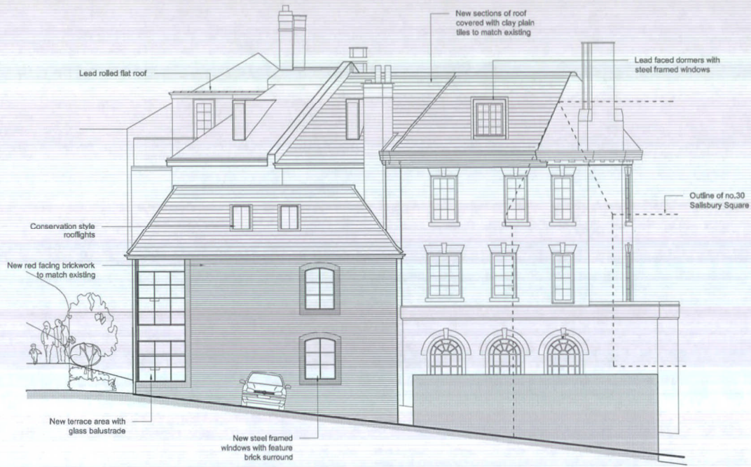
South Elevation (from car park) scale 1:100
