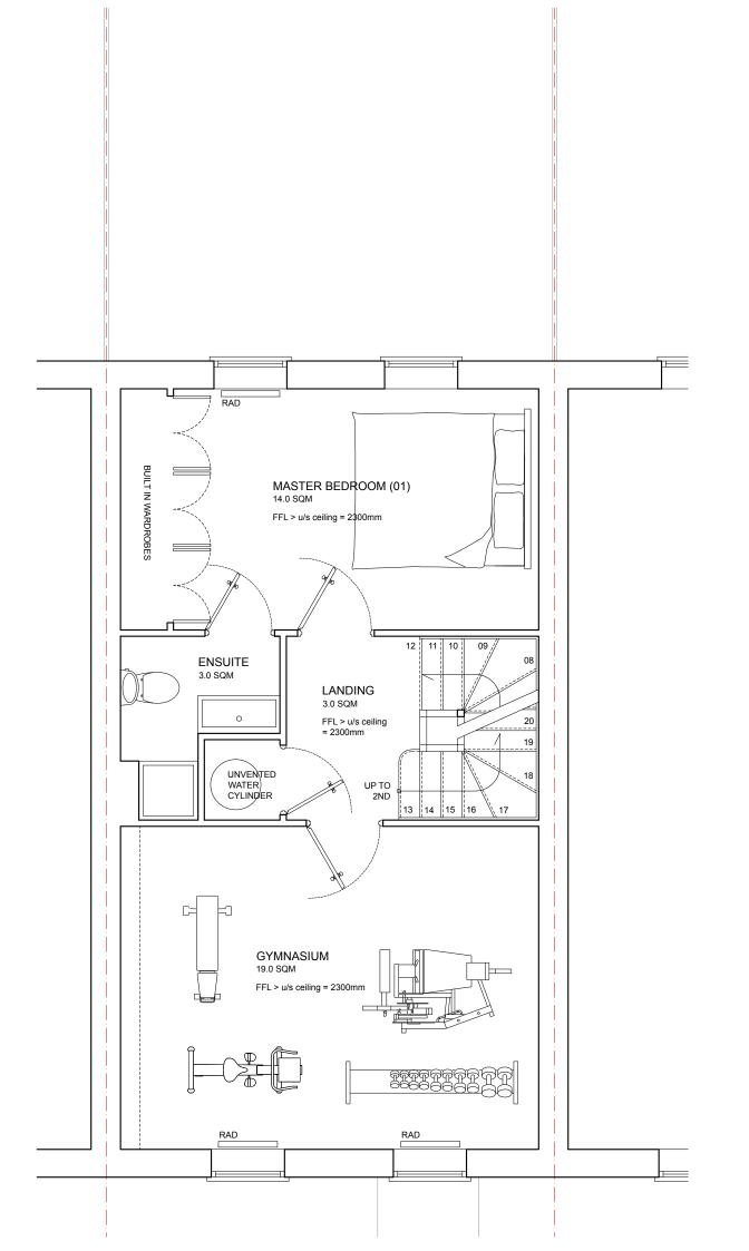
**EXISTING FIRST FLOOR PLAN** SCALE 1:50
