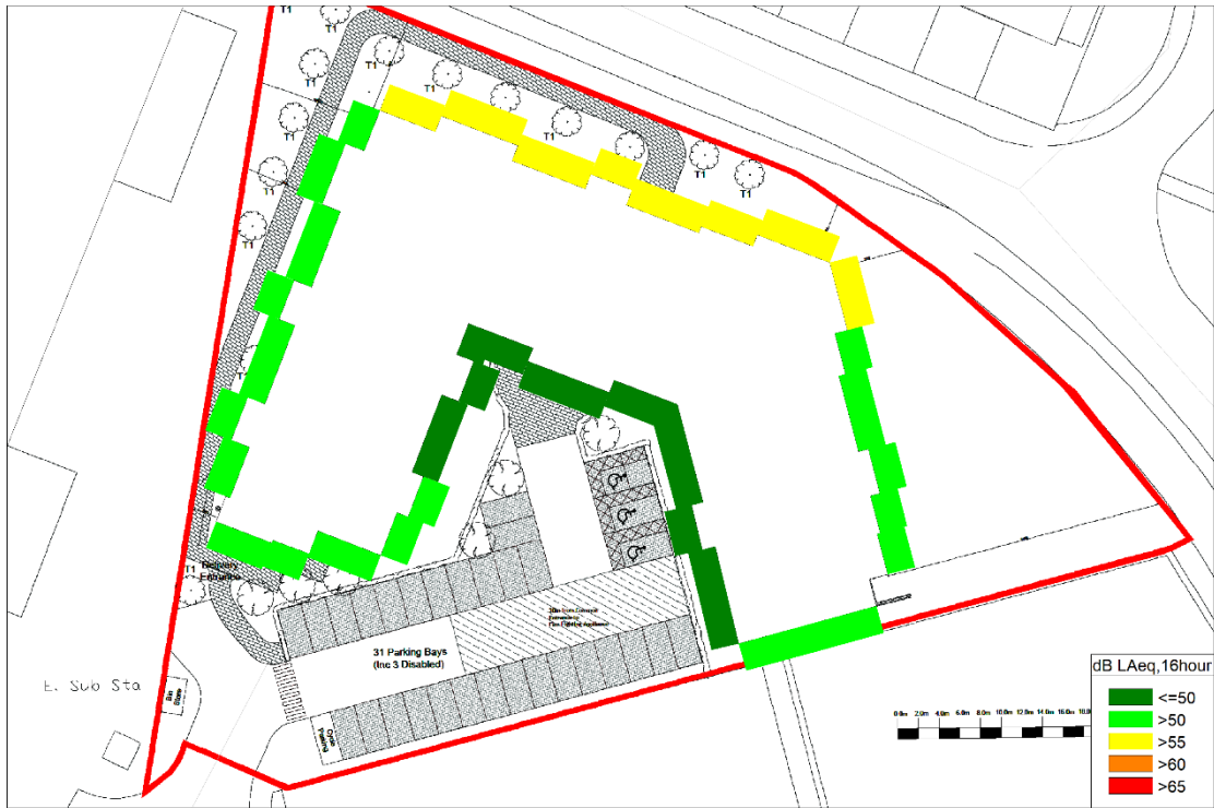
Figure A1: Daytime façade noise levels (dB L_{Aeq,16hour} )
