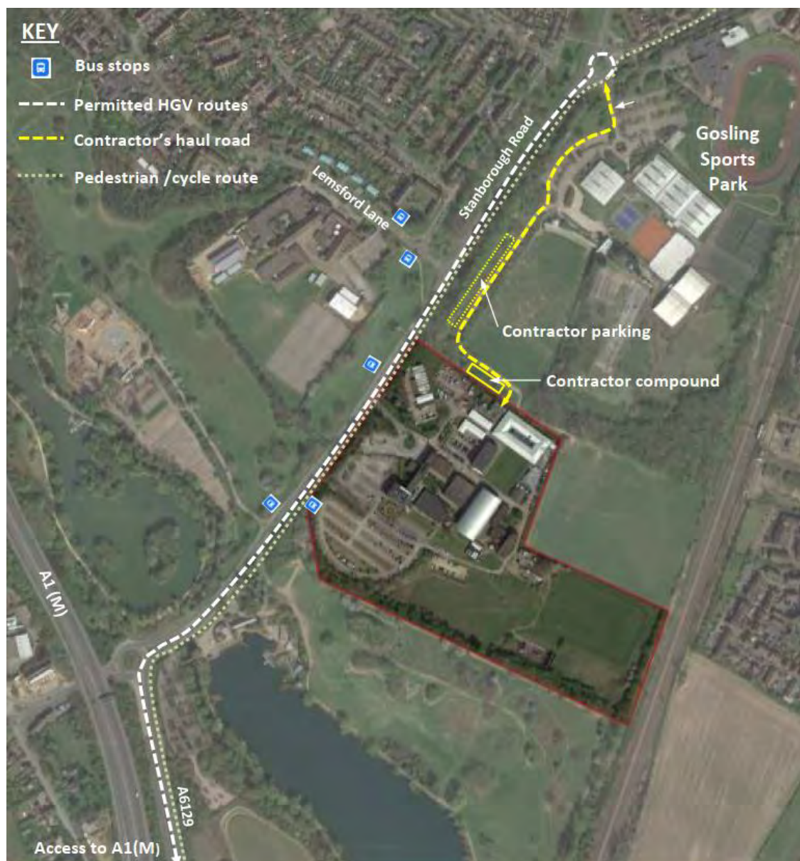
Figure 4-5: Proposed Construction Vehicle Access Route
