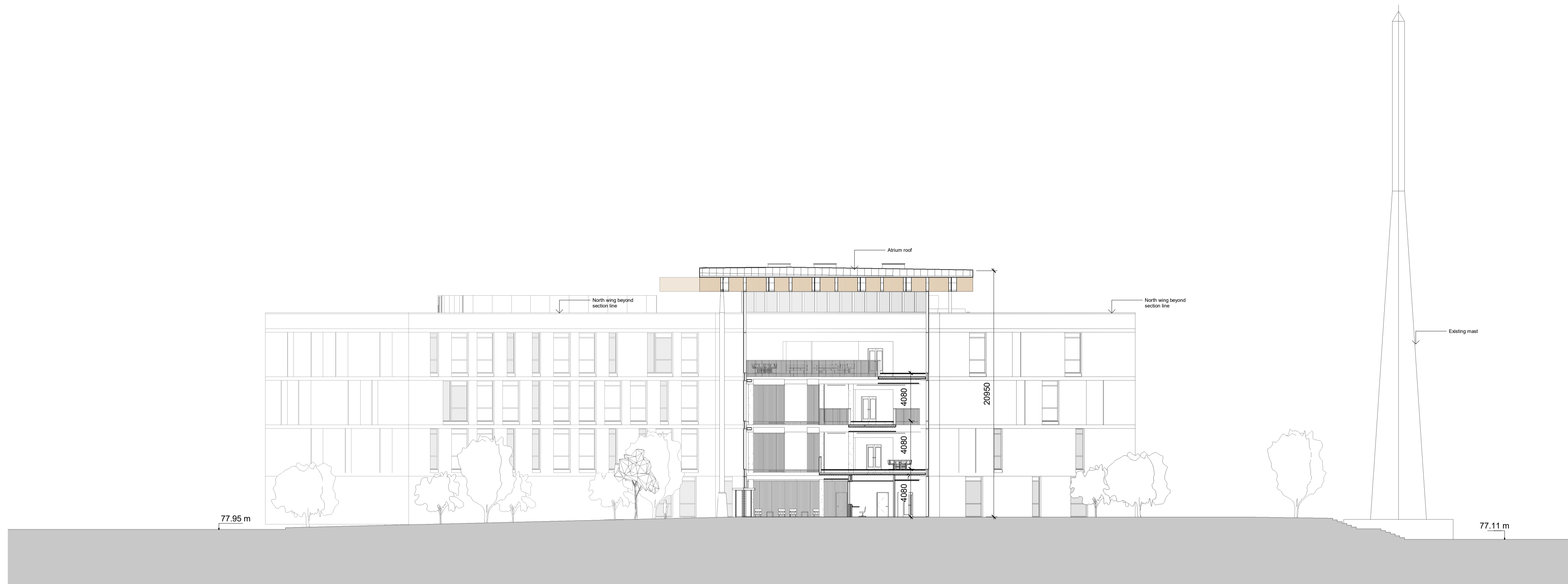
Section A - Atrium Cross-Section 1 : 200
