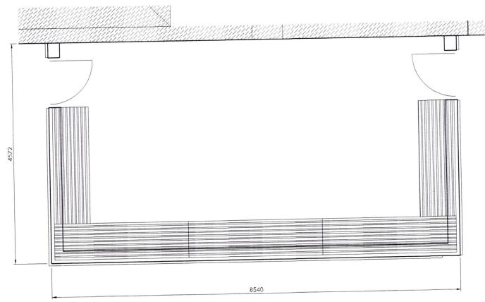
'Victorian' lean-to greenhouse Masonry base and rear walls (existing) with new painted timber and aluminium glazed superstructure
