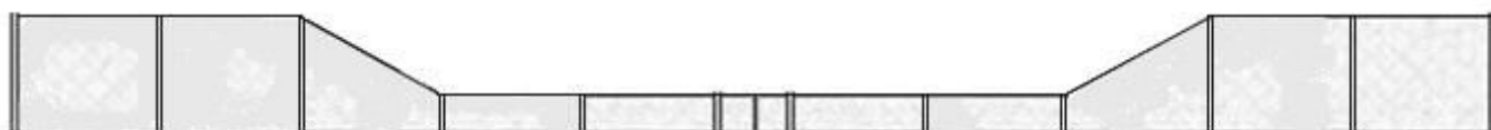
West Side Elevation – Length 35 metres – Height ranging from 2.75 metres down to 0.9 metres
