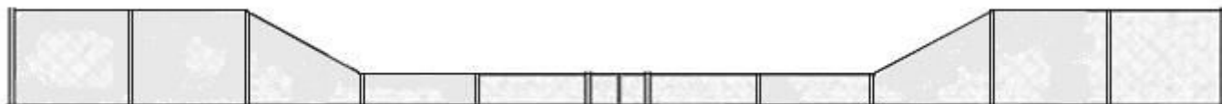
East Side Elevation – Length 35 metres – Height ranging from 2.75 metres down to 0.9 metres
