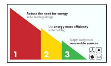
The principle of the energy hierarchy is demonstrated by the diagram below:
