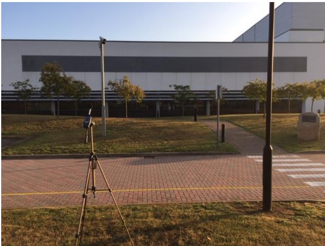
Photograph No.3 & 4. Position #2, South perimeter (adjacent to the access gates), alongside 'Tablin Way' and opposite the departments (dwellings), well away from the factory building or any other noise reflecting features.
