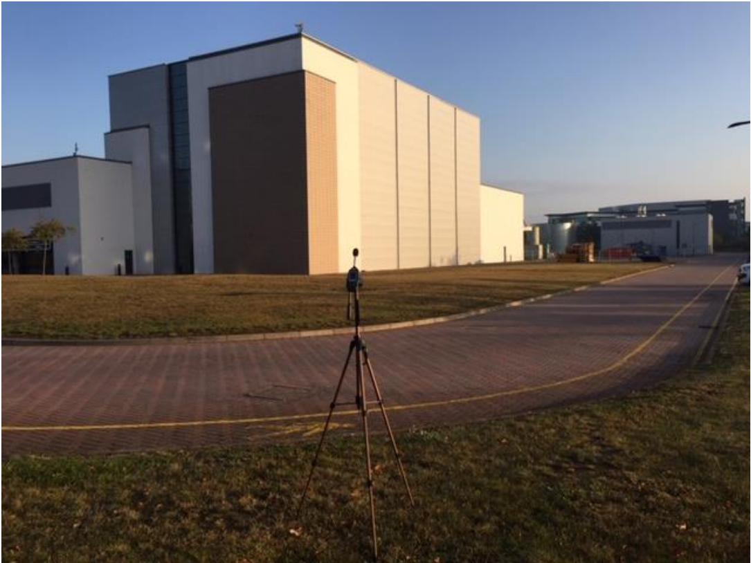
Photograph No.1 & 2. Position #1, South East corner of south perimeter, well away from the factory building or any other noise reflecting features
