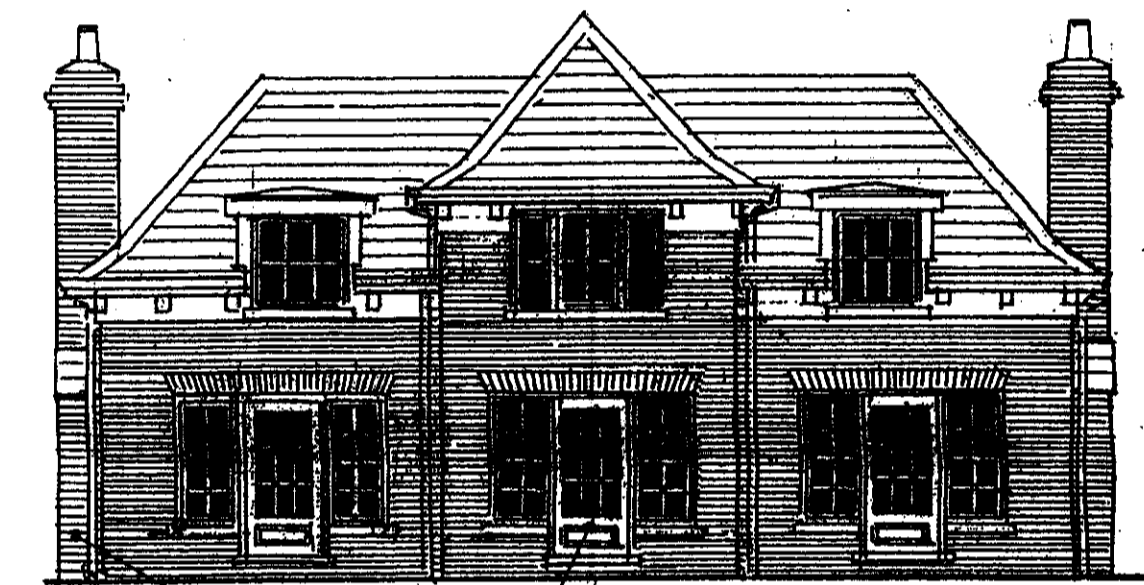
Revision 'A' Proposed additional chimney stack and alteration to fenestration NORTH WEST ELEVATION
