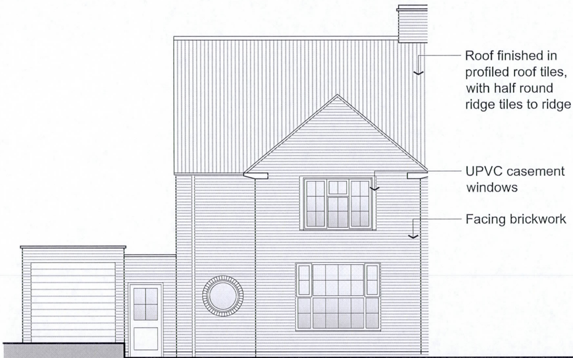
Existing west elevation SCALE 1:100 at A3
