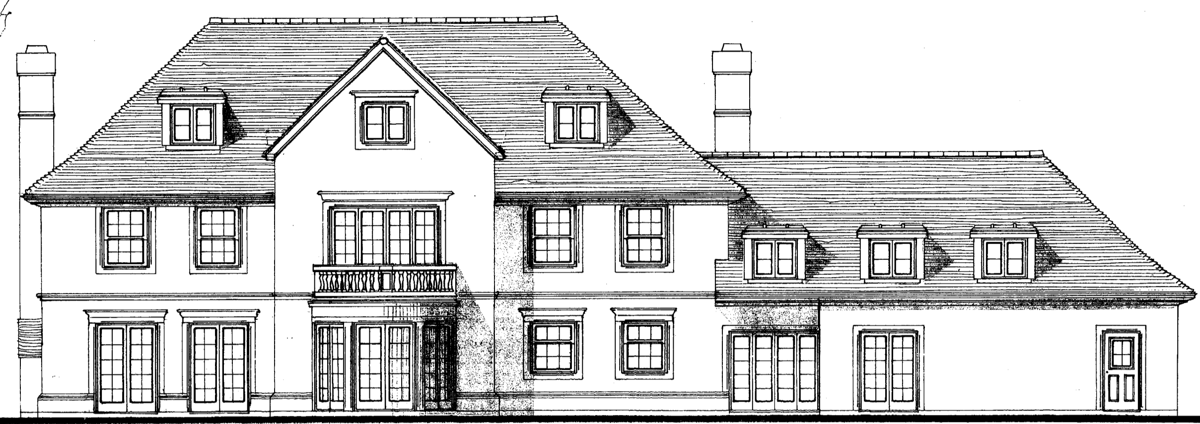
EAST REAR ELEVATION Straight segmental glass panels to balustrading to curved bay to dining room with master bedroom balcony above
