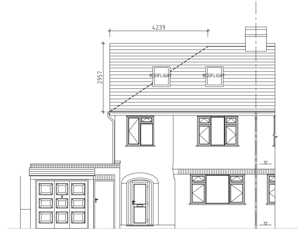
FRONT ELEVATION - PROPOSED - Scale 1:100
