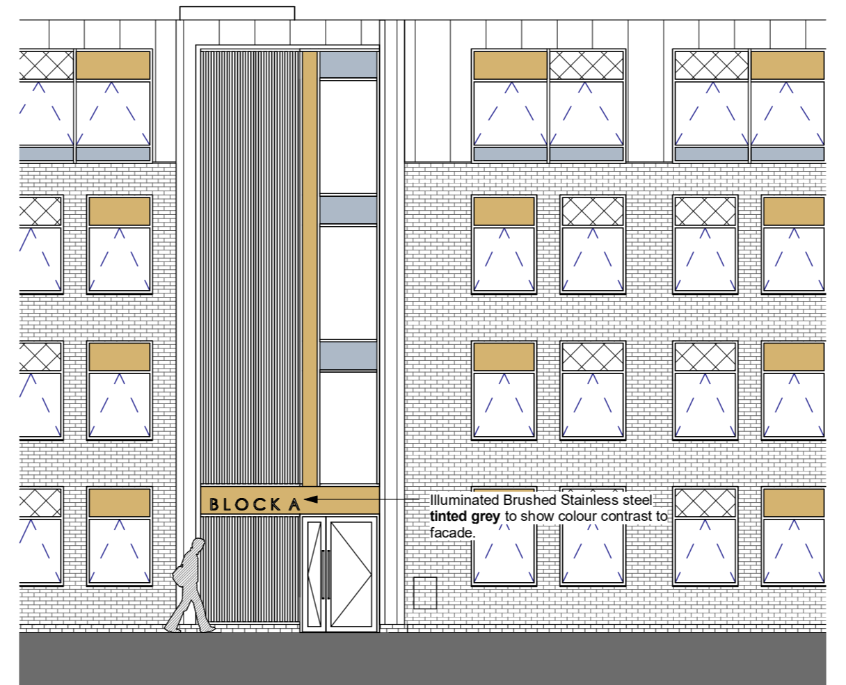
B. BLOCK A - External signage East Elevation (TYPICAL TO BLOCKS A TO F) 1:100
