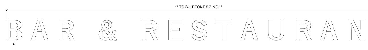
Signage to maintain appearance in keeping with 'THE COMET' orignal illuminated signage. Font is Yu Gothic Sign to be built up PPC stainless steel lettering with open stroke, to have internal face permanent illuminated lettering to the same profile. Internal letters to have white opal acrylic faces and internal premium white GE LEDs to create even face permanent illumination. This specification matches all other external signage currently on the building.
