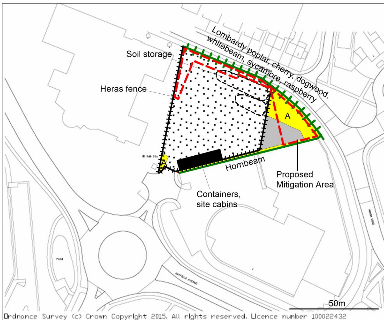
Figure 10 – Phase 1 habitats (JNCC 2010 categories) at Hatfield Avenue, Hatfield: Bare ground (black dots on white), Amenity grassland (yellow, labelled 'A'), Hardstanding (grey), Intact species-poor hedge and trees (green hatched line), Intact species-poor hedge (simple green line), Buildings (black), Fence (black hatched line). Two soil storage mounds are marked (black dashed line), and a proposed Mitigation Area is shown (red dashed line).
